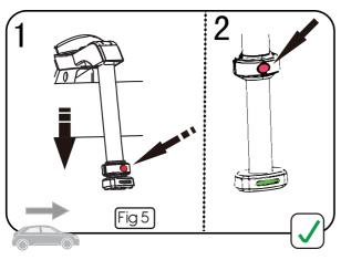
Press in the foot release button on the bottom of the leg to extend the foot until it is in contact with the floor of the vehicles footwell. Fig 5.
