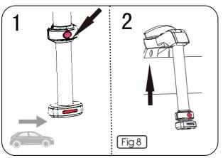
Press in the bottom on the leg and retract the foot. Fig 8.
