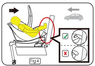
Press in the small ISOFIX release button and push forward on the car seat until it touches the back rest of the vehicle seat. Fig4.
