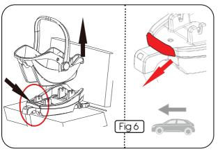
Put the carrying handle of the car seat into the carrying position. Pull backwards on the Isofix lock catch until the window is showing red. You can now lift the car seat away from the base. Fig. 6.
