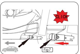
Pull sideways on the black ISOFIX points until the window is a red colour to unlock the Isofix base from your vehicles Isofix fixing points. You will hear an audible click when this is done correctly. Fig 7.
